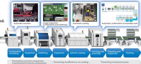
Eliminating shipping of defective solder by machine inspection
